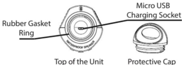
The Micro USB charging port is located under the Protective Cap. Unscrew the Protective Cap in a counter clockwise motion to gain access.
